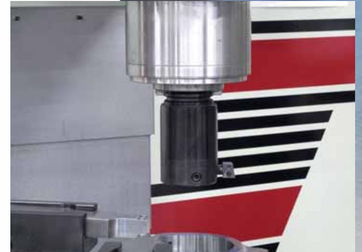
Connecting Rod bore tooling installed in massive F68A spindle.
