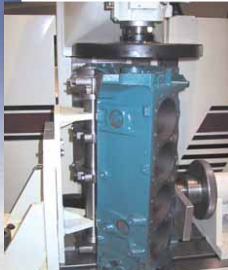
The block end truing fixture quickly attaches to the 4th axis rollover fixture or the precision performance fixture for exact alignment of transmission and engine block. Dowel truing for centralizing transmission and crankshaft centerline
