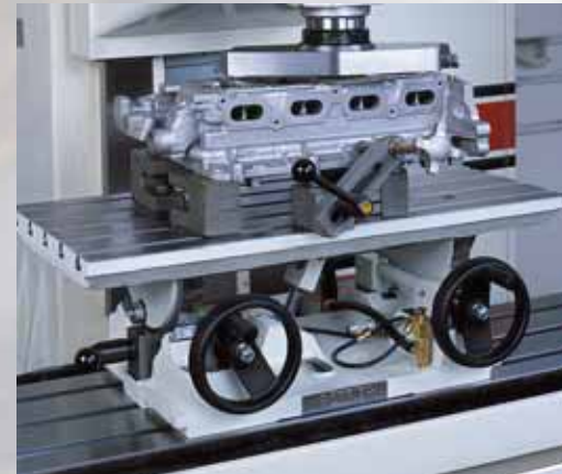
Rottler's patented 2 axis leveling table and universal quick clamping system for surfacing/ milling heads, blocks and manifolds with CBN and PCD tooling.
