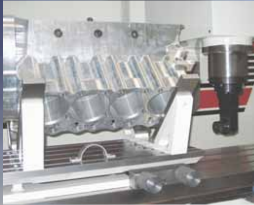
Rottler's new pivot table allows quick set-up for line boring.
