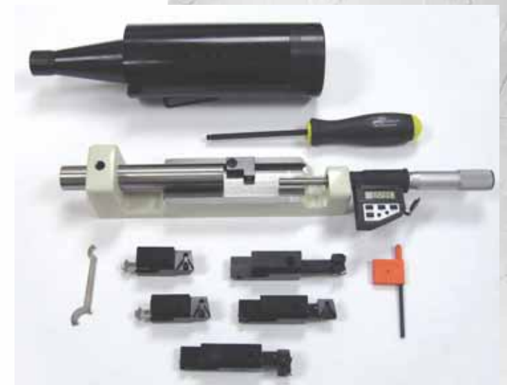
Boring and Sleeving Cutterhead, tool holders and Digital Setting Fixture
