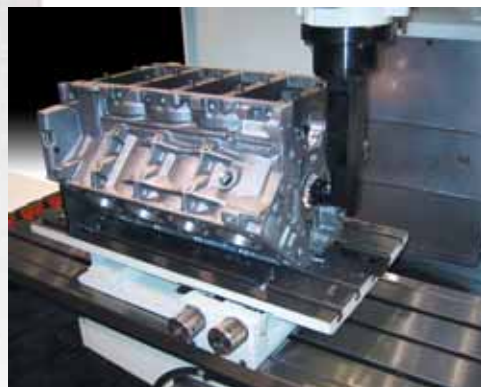
Cam tunnel modifications and roller bearing conversions. Some blocks allow main and cam line to be bored in one set up with extended slim line right angle drive.
