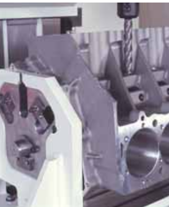
Lifter bore angles are accurately set with gage blocks in the Performance Fixture. Complete a lifter bushing job in less than one hour!
