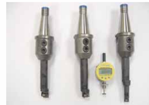
Single point Lifter Tooling and digital setting fixture for boring, facing and finishing lifter bores and bushes.
