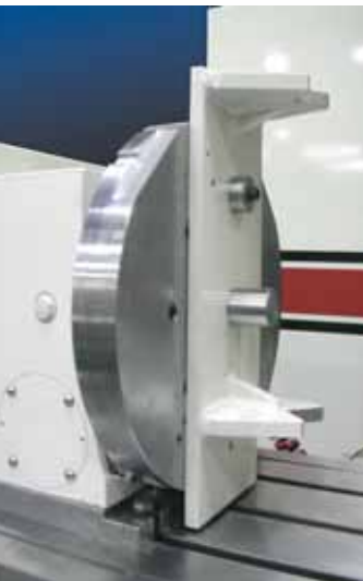
The block end truing fixture quickly attaches to the 4th axis rollover fixture or the precision performance fixture for exact alignment of transmission and engine block. Dowel truing for centralizing transmission and crankshaft centerline
