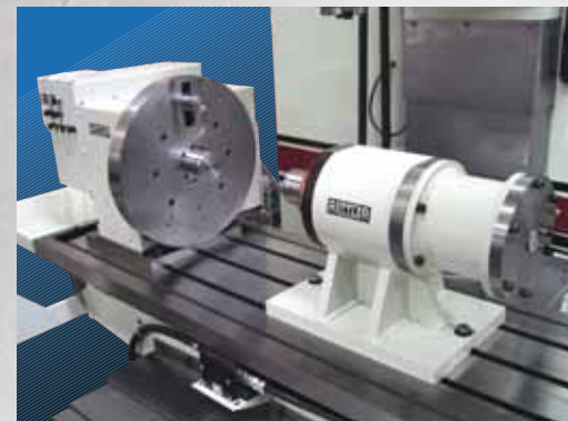
Rottler's NEW Universal Quick Load/Unload Automatic Rotate 4th Axis Fixture and Software allows the control to rotate the block or cylinder head during the automatic machining cycle.
